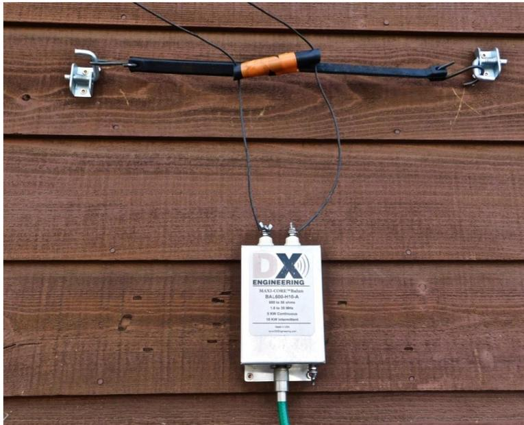
Using a Cottonwood tree and a 30-foot tower he just put up, the antenna ends are nicely positioned East/West. A 600 Ohm ladder line feeds the antenna at center then goes to a Balun {600 Ohm : 52 Ohms}, then coax into the shack.
