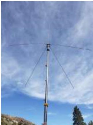
I used this resource: (<https://m0ukd.com/calculators/quarter-wave-ground-plane-antenna-calculator/>) for radial lengths and tuned this for 146.520 Mhz. After preliminary testing, I get near perfect 1:1 SWR across the 2m band and acceptable SWR on 70cm, although it is more variable in the later.
