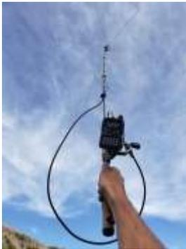
This design relies almost entirely on the very common 1/4 Quarter Wave ground plane based on the SO-239 chassis connector. I made a few additions to this in order to make the antenna easily assembled/disassembled and able to be hoisted several feet above one's head if needed. A high priority was put on its ability to be stored easily while in transit via backpacking.
