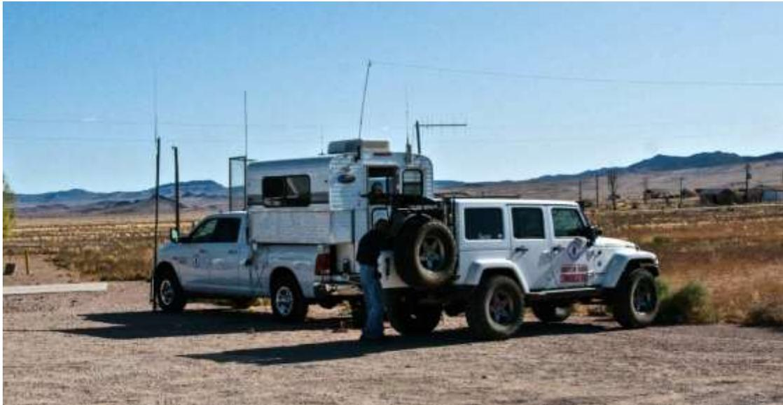
We set up three local HF radios, one for 3965 KHz, one for 7280 KHz, and one for Digital communications on a number of frequencies using the long wire antenna. We used a fourth radio located in Las Vegas that was operated using an Internet link from Rachel. We didn't know if there would be LTE available to provide an Internet connection, but it worked throughout the entire operation and we used that radio both on HF and on VHF in the Las Vegas area.
