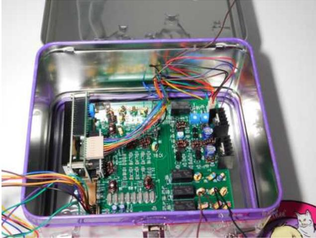
Radio sitting in lunch box. Sizing for where to drill for the display, knobs (on left) and the antenna BNC (two wires at lower right). Board will end up being mounted about 1 1/2" to left. LCD display will poke through the left side of the box.
