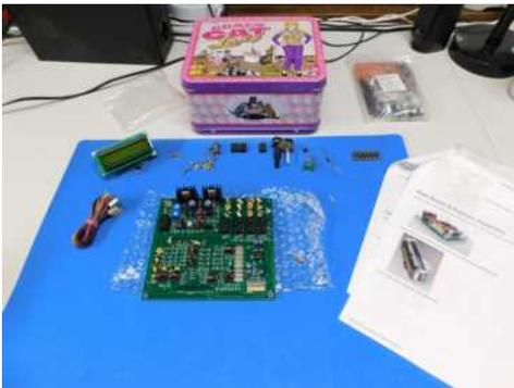
Entire kit laid out. Blue cover is an anti-static mat. HF multi-band radio, QRP, SSB and CW. Lots of hams have created add-ons, including a small board to add digital capability.
