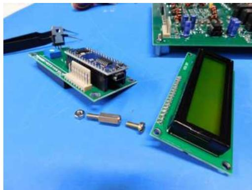
Rudiono on left, attaches into sockets on the display, shown on right. Main board in background.
