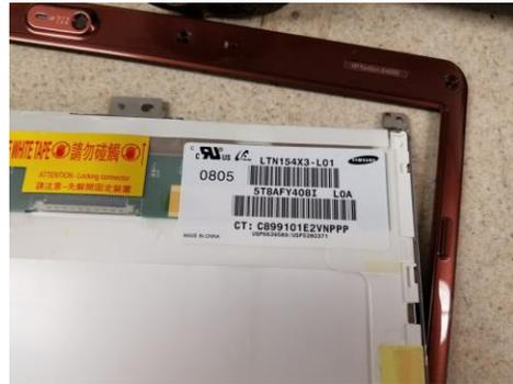
All that was needed to get the correct controller board was to take the screen from its case and find the brand and model on a sticker on the back. This ensured the correct cabling for a plug-n-play connection.
