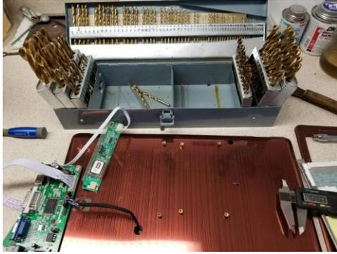
I drilled holes in the aluminum monitor cover and used motherboard stand-offs from my computer parts junk box. It seems solid and works for now. The standoffs threaded right into the aluminum case. All that was necessary was the correct size drill bit.
